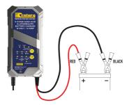
Connect the Red (+) Crocodile clip or ring terminal to the (+) battery terminal. Connect the Black (-) Crocodile clip or ring terminal to the (-) battery terminal.
